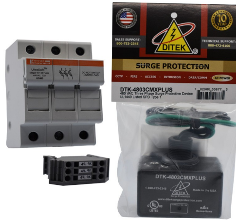
480 VAC Phase Monitor Kit Part # DFS-00393-008-05 (Kit includes 480 VAC, three-phase surge arrester, three DIN-rail mounted terminal blocks with integrated 49.9k resistors, and fuse block with three 1 Amp fuses)
