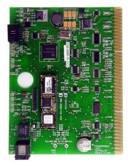
enables the PLC800 to function as a network slave device using either DFS NIM RTU protocol or Modbus TCP protocol. The PLC800's serial port enables it to function as a Modbus RTU/ASCII master or slave device.
