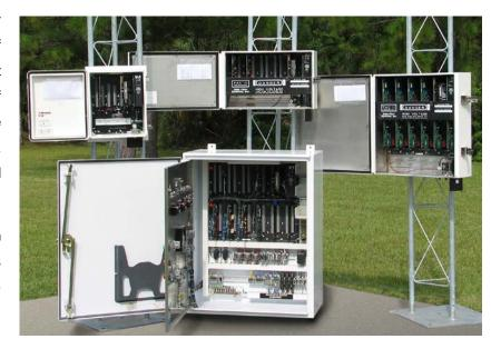
The 200 Series RTU is available in four models with each offering a variety of mixed digital and analog input and output RTU I/O modules for an extremely versatile solution. A DFS PLC module with an optional Panel PC is utilized for automation and process control applications. Powering by 120V or Solar is available. Typical RTU communications are by FCC licensed radio frequency, and/or IP Network is offered (supports dual-mode communication). Cellular SCADA is also available.
